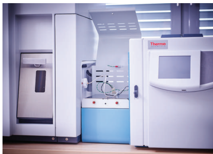
Figure 1. Coupling is achieved by connecting the GC column directly to the ICP-MS torch using the GCI Series Interface.
