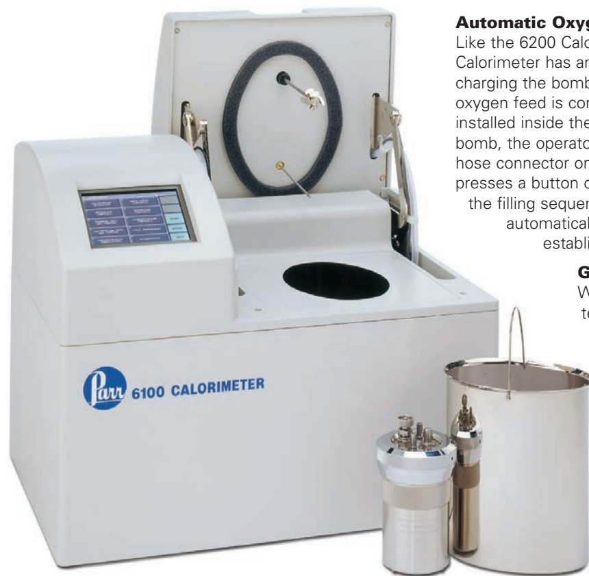
6100 Calorimeter open with 1108P Bomb and Bucket
