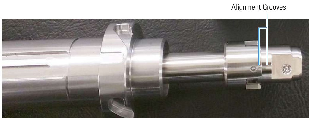
Figure 29. Attaching the V-lock Source Plug to the Source Exchange Tool
