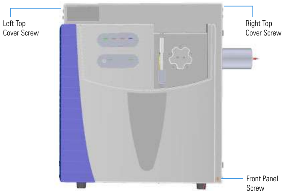
Figure 1. Hydrogen Safety Screws on the Mass Spectrometer
