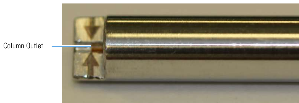
Figure 24. Lining Up the Column in the Column Measuring Tool
