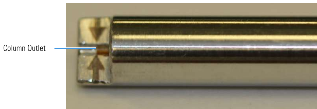
Figure 17. Lining Up the Column in the Column Measuring Tool
