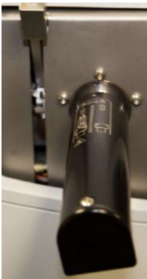
Figure 31. V-lock Source Plug Inserted Correctly
