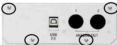
Fig. 9: Screws on the access panel
