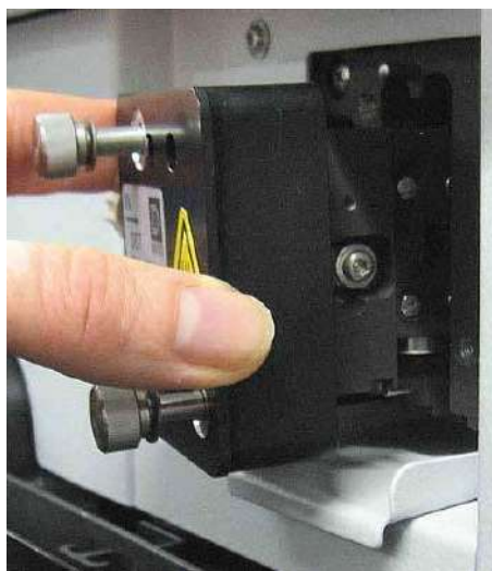
Fig. 17: Inserting the flow cell
