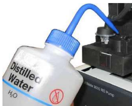
Fig. 19: Filling water into the connection port
