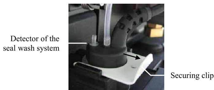
Fig. 18: Detector of the seal wash system
