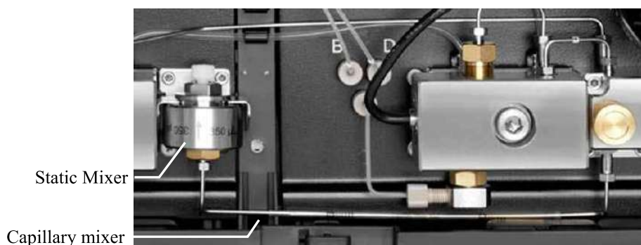
Fig. 5: Two-step mixing system (here in an HPG-3400SD)
