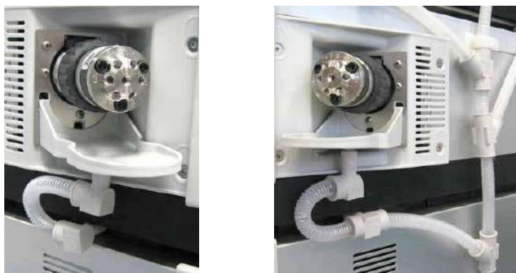
Fig. 16: Drip tray with drain tubing connected to the left valve and to the right valve
