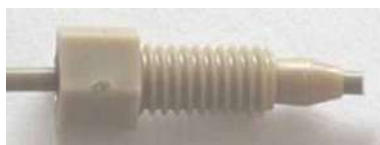
Fig. 25: Capillary with fitting screw and ferrule for connection to the biocompatible valve pod
