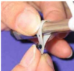
Fig. 20: Attaching the column ID to the column
