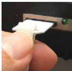
Fig. 41: Inserting a column ID chip card in a chip card reader
