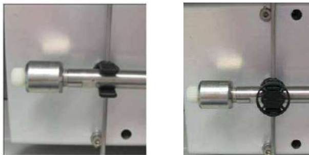
Fig. 21: Installing a column in the clip
