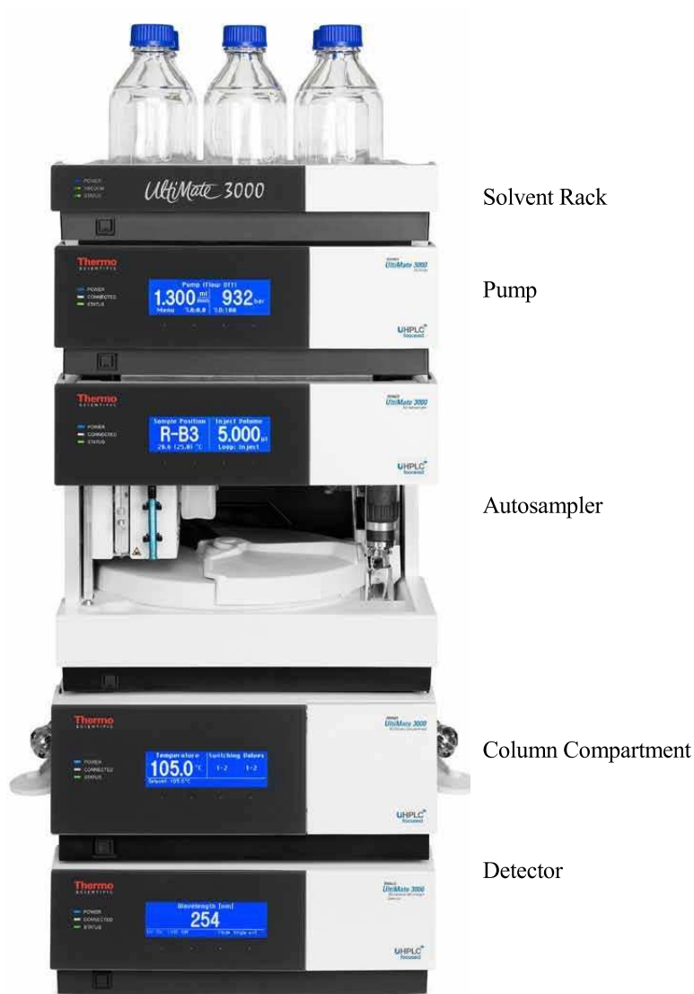
Fig. 7: Module arrangement for an UltiMate 3000 system (example)
