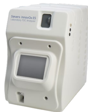
Figure 1. Sievers* InnovOx Laboratory TOC Analyzer used to measure the spiked condensate samples
