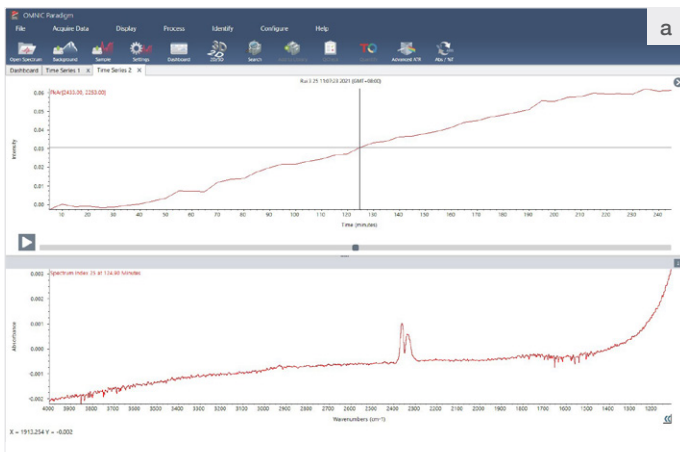
Figure 2. (a) Representative CO 2 peak area profile and FTIR spectrum of an accelerated ageing test; and (b) 3-D representation of an accelerated ageing test. The area inside the red rectangle shows the CO 2 evolution over the course of the experiment.
