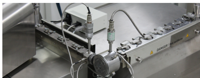
Figure 1: Setup of twin-screw extruders for co-extrusion.
